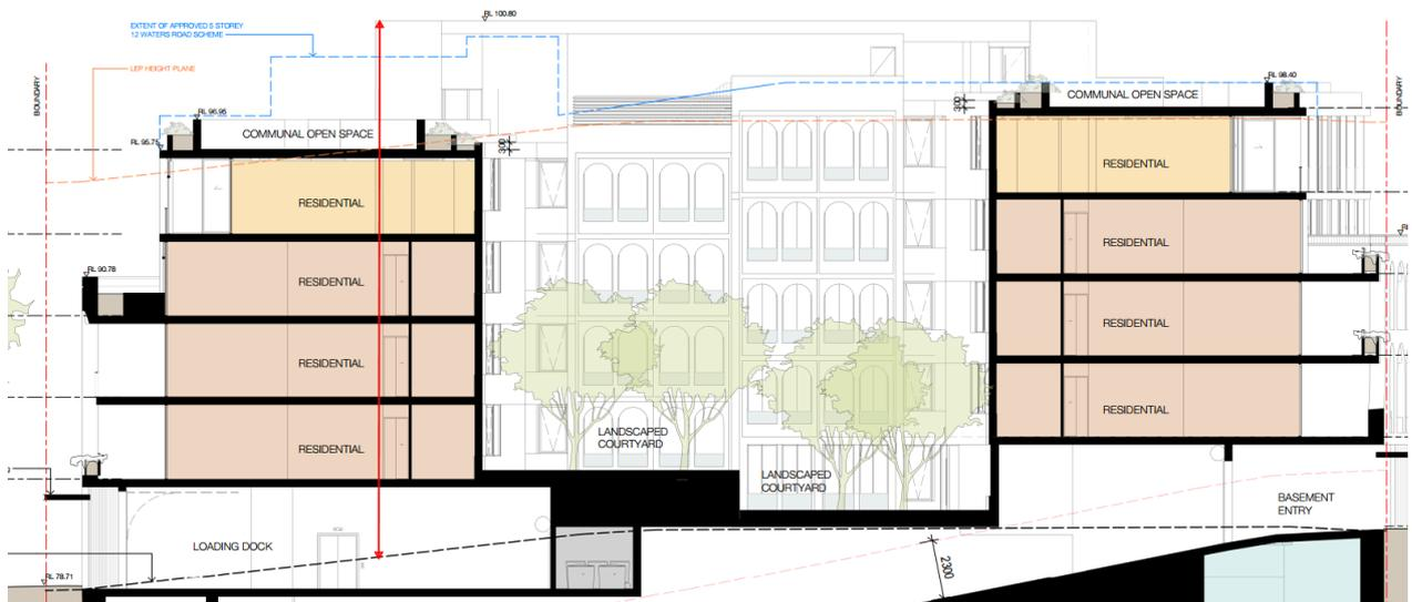
Figure 2: Extract from architectural section drawing DA-0601 - Vertical red line showing the maximum building height of the proposed development
